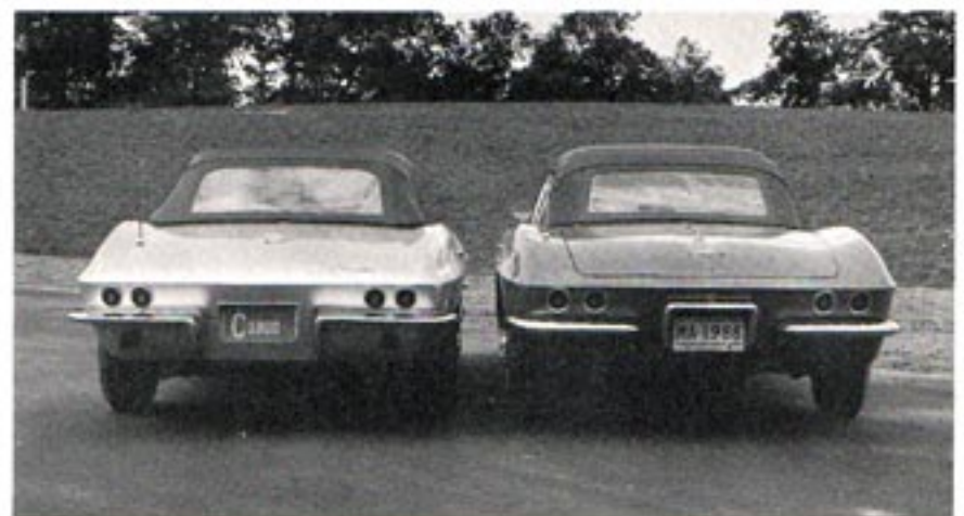
Figure 2. Decreases in overall length, width and height contribute to the small silhouette appearance. The passenger compartment of the 1963 Corvette is moved rearward and the wheelbase shortened.
