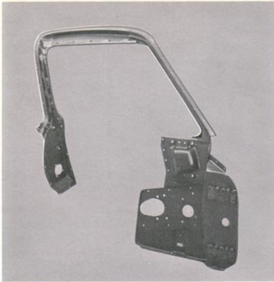
Figure 10. Door steel reinforcement.
