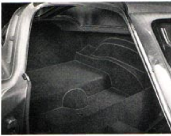
Figure 5. Below the removable floor panel are two depressed areas, one on each side of the tunnel. The left hand space is utilized for tool stowage.
