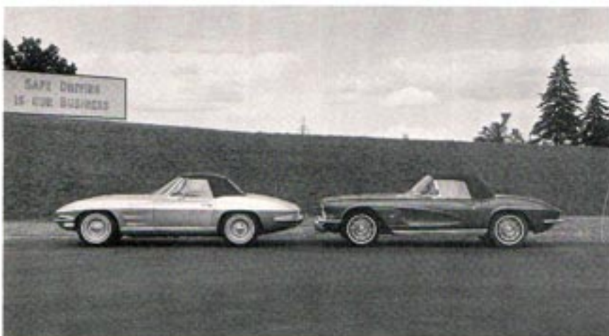
Figure 2. Decreases in overall length, width and height contribute to the small silhouette appearance. The passenger compartment of the 1963 Corvette is moved rearward and the wheelbase shortened.
