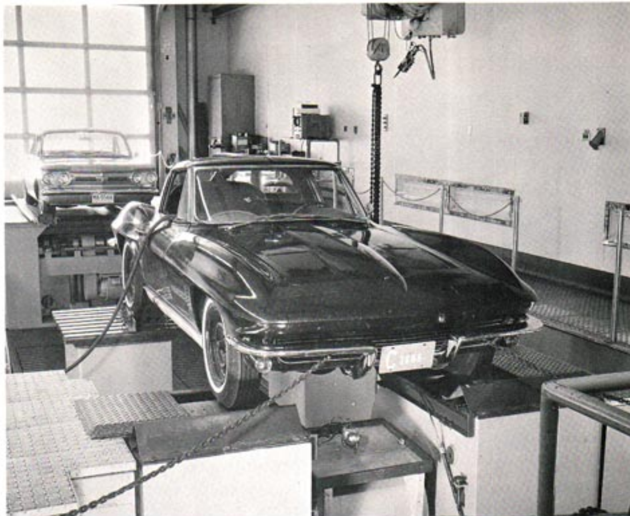
Figure 17. Complete vehicles were tested on the chassis rolls to determine the dynamic characteristics of the body and frame combination.
